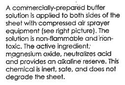
Once the buffer is applied, the paper's pH alters slowly. After deacidification, random testing ensures an 8 pH with a deviation of no more than 2-4%.
